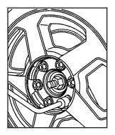
4. Use the wheel wrench to tighten the nuts firmly. Try to move the tire back and forth slightly to be sure it is secure.
